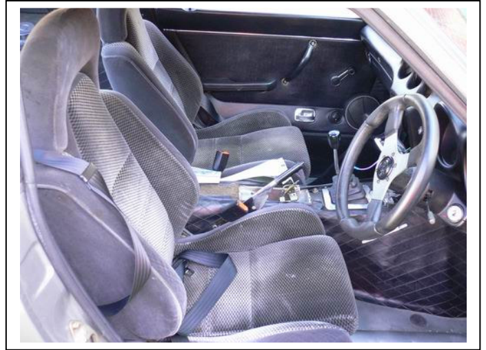
The new driver seat, much more comfortable, supportive, with adjustable height, lumbar support and ability to tighten the back side supports to suit your back width & cornering speed!!
