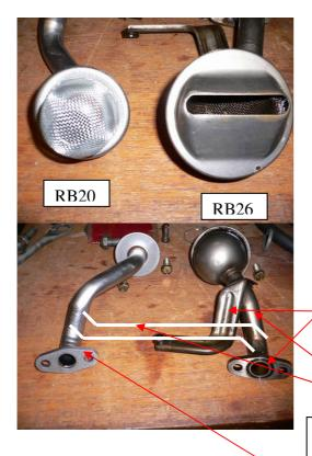
The original RB26 oil pickup on the right and the RB20 pickup on the left See the O Ring on the RB26 pickup
