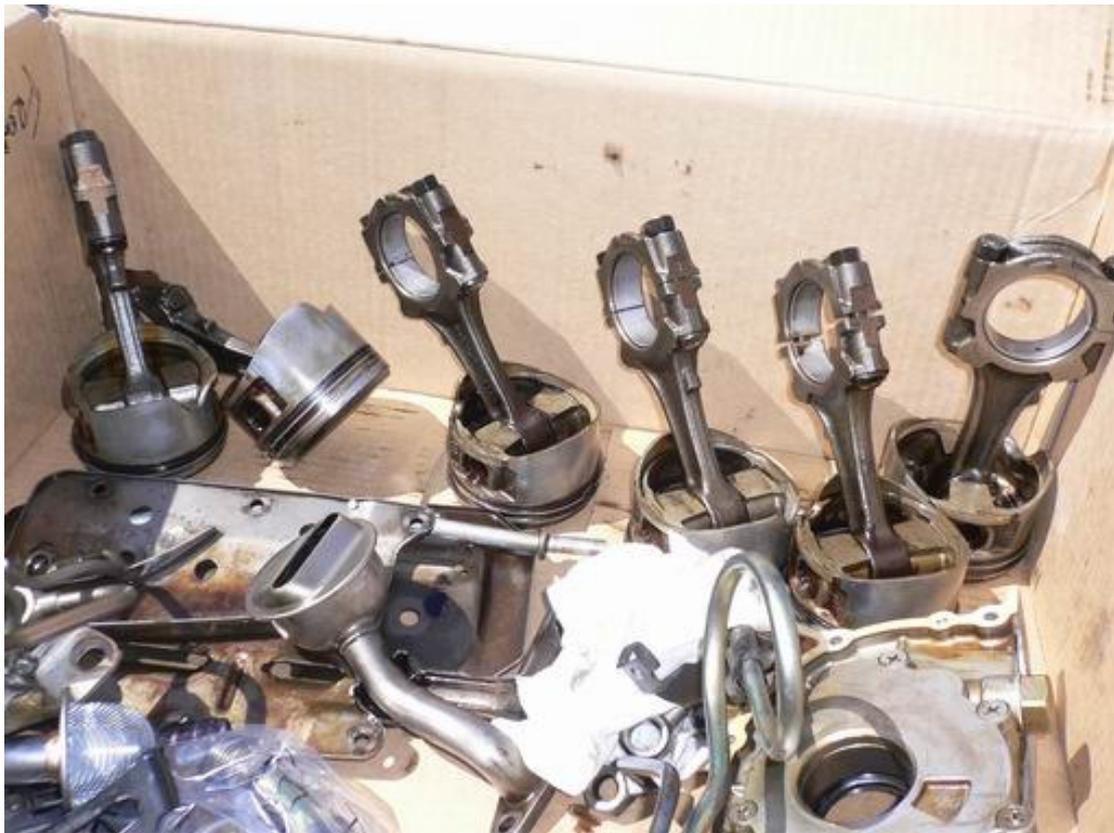
Six pistons as removed from the motor in prep for the block testing
