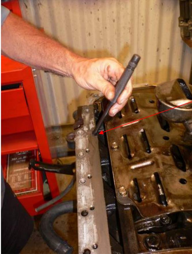
Drifting out the dipstick from the front original position
