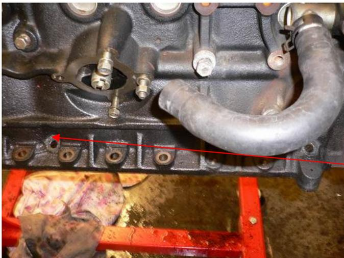
Dipstick now removed from front awaiting removal of brass plug from rear
