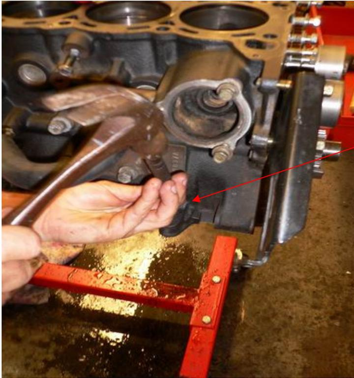
Drifting in the brass plug to the front dipstick hole
