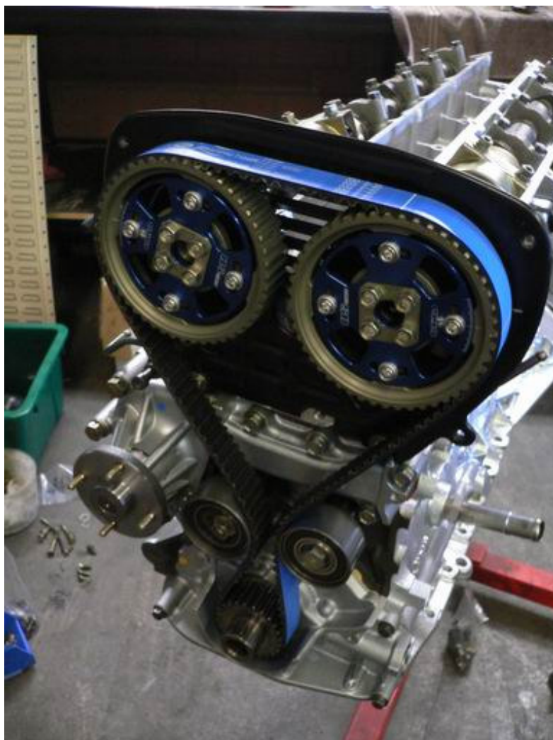
New Gates timing belt in place
