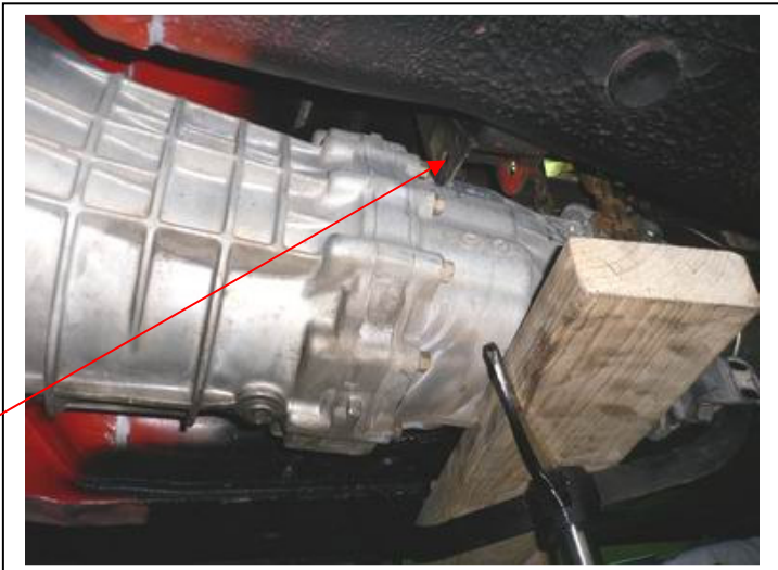
The RB25DET gearbox, showing where it fouls the original gearbox mount "ears".
