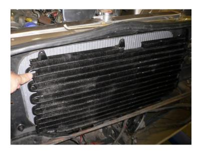
The Europa condenser fits in easily but the pipe routing is in the way and it is old.
