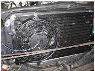
The skew bladed condenser fan \$148 fitted in well, and was bolted to the radiator shroud.
