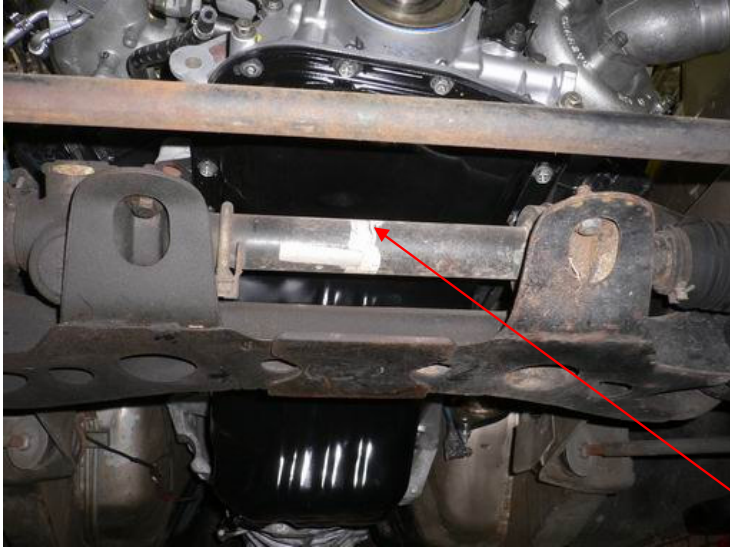
The RB20 sump clears the sub frame and the steering rack well
