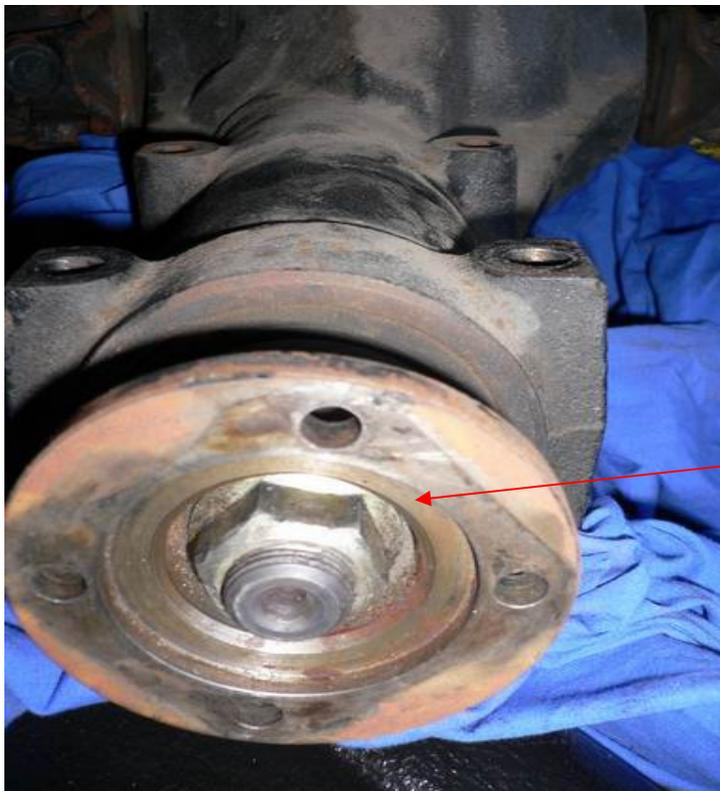
The R200 diff that was in the car – 58mm coupling, rather than the 50mm coupling of the Z31 R200 LSD
