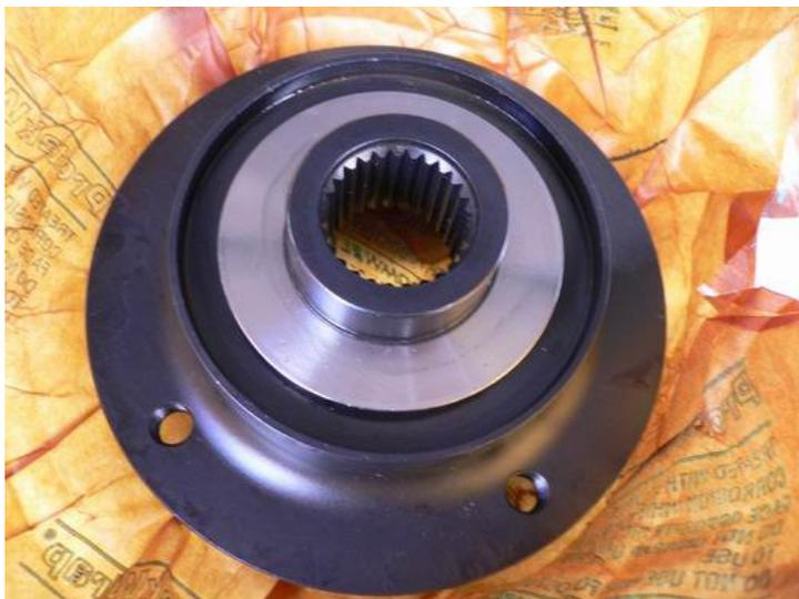
Billet companion flanges & fittings supplied by Ross at Modern Motor Sports in Canada. These are to allow the CV joints to be fitted to the 240Z. They are well made, and we are lucky there are people like Ross and John Coffey (camber plates Part 16) around that make all these things possible.
