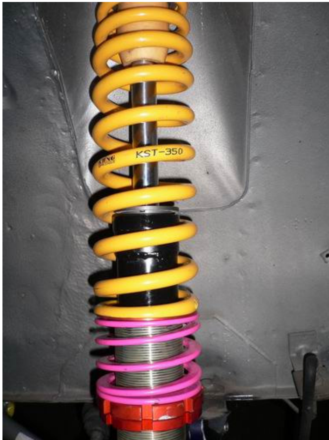
350lb progressive springs in front & Koni shocks
