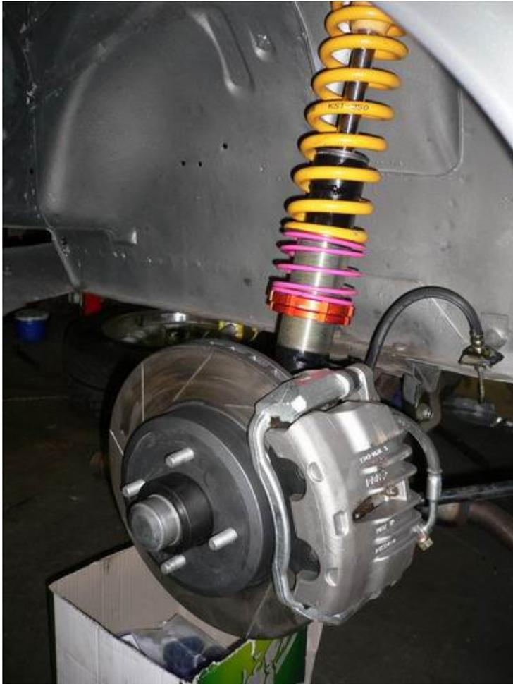
New 300mm rotors & callipers fitted to new adjustable struts, all bled and ready to go
