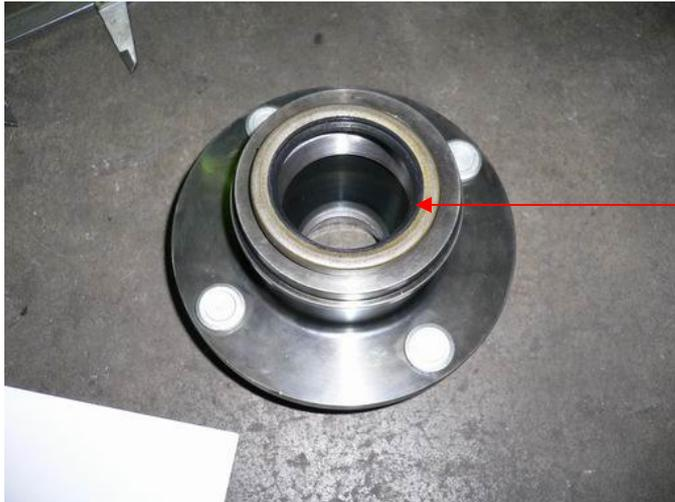
The seal is 2mm bigger than the machined hub
