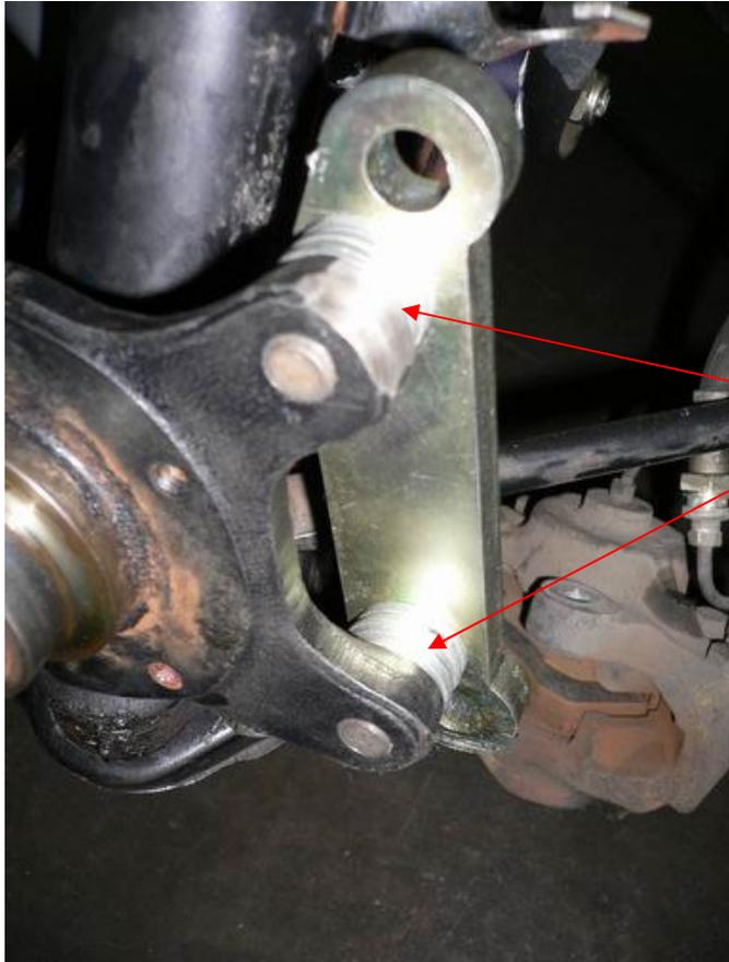
The calliper brackets had to be shimmed up with washers and then a solid spacer piece made. I later found out that Hopperstoppers do supply two billet spacers in the kit.
