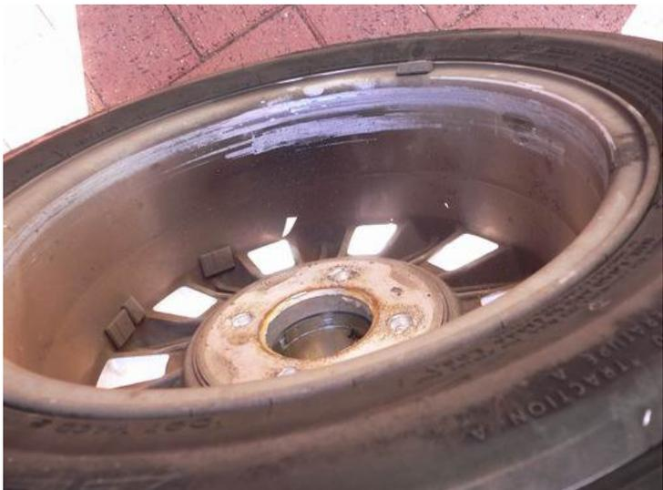
Oops – the wheel won't bolt up clearly! The calliper scrapes on the inner edge of the wheel in a band about 35mm wide.
