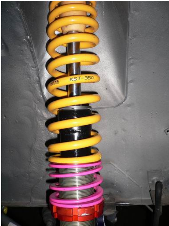
350lb progressive springs in front & Koni shocks
