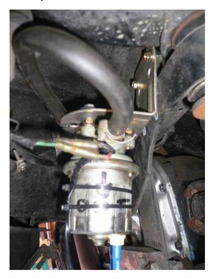
My webber tuner Barrie, advised me to change the fuel pump to this Carter pump, which whilst very noisy does the job. Mounting it on rubber may help - a job for me to fix later.
