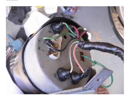
After fitting the Crane Hi Power coil and management system the tacho then wouldn't work.
